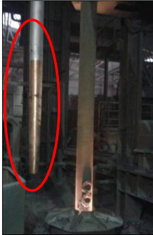
Figure 7 - First Slagless® AM JM before first blow and peculiar cartridge face.
