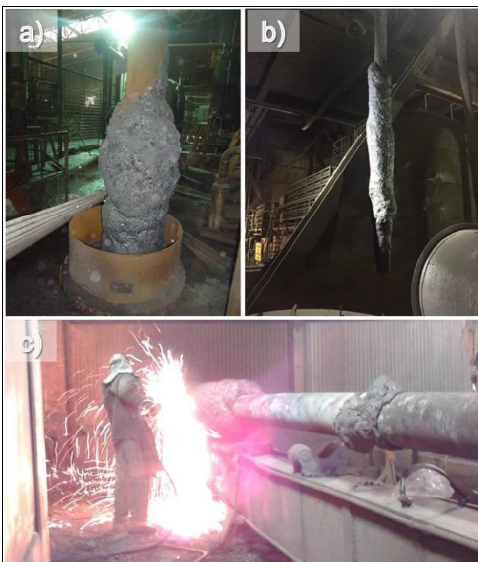
Figure 4 – Scrap formation at conventional lance and tip face. a) Represent the scrap lance during domo passage and b) Represent the scrap extension along lance length.
